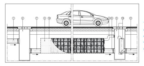
The flow may be regulated by a nozzle arrangement (a calibrated orifice), by a limiter based on a vortex effect, or by a guillotine-type regulator.
