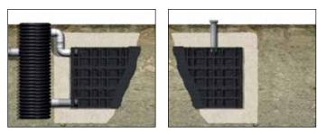
Vents must be used to regulate the pressure levels inside the structure and provide it with ventilation.
