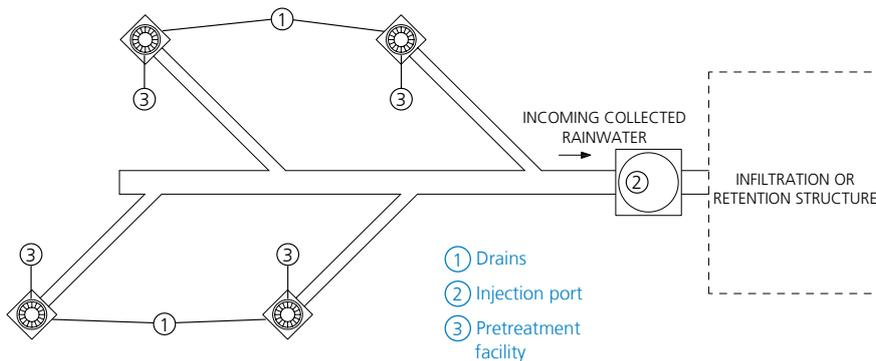
This kind of offset arrangement for pretreatment may be achieved with a honeycomb cartridge filter (with the capacity adapted to the flow rate for a structure with a single collection facility).
