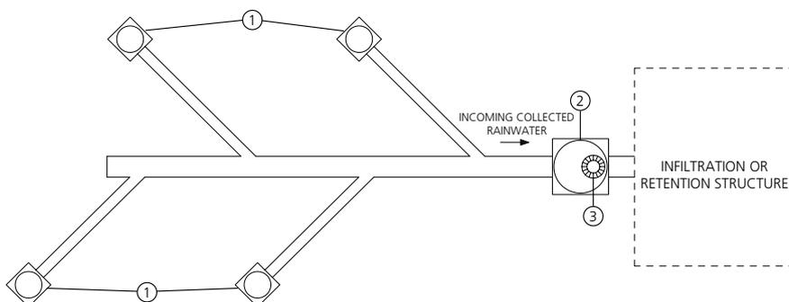
This kind of centralised pretreatment may involve a circular filter with a high flow rate (capacity adapted to the flow rate for a collection structure).
